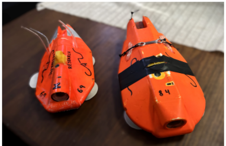
Suction cup tags used to study Rice's whales. Credit: NOAA Fisheries/Meaghan Emory
